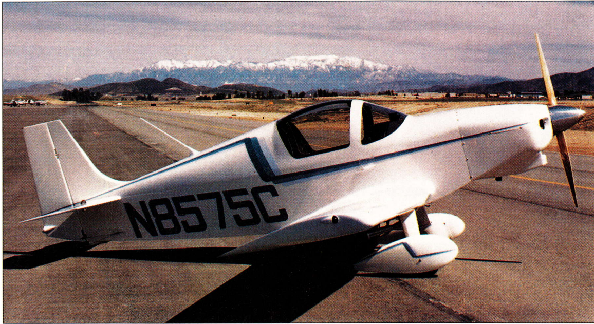
Richard Lind of Santa Paula, California, designed his own canopy for his KR-2.
