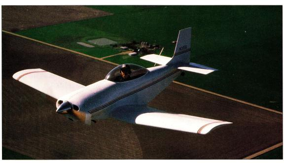
and cost only \$1500 to build back in the mid 1980s. He started out with a \$500 investment in a damaged KR-1 that contained complete metal fittings and other usable components. The 49-year-old builder pioneered the fixed-gear version. Shirley admitted that his gear design was influenced by the RV-4 and constructed it out of 7025 T-6 aluminum. He also made his own wing design, a wing that was 2 feet longer than the plans and tapered from 4 feet at the root to 2 feet at the tips for speed.
